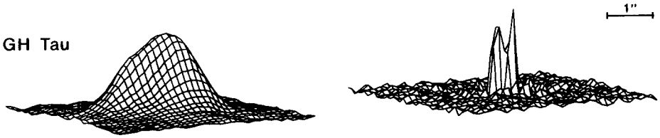
Fig. 16. Gain in spatial resolution obtained by speckle interferometry at 2.2 \mu\text{m} on an object with a K brightness of 8.3 mag. Left: Long exposure image, the seeing at K was \approx 2.0'' . Right: The image reconstructed from the same data by speckle methods. It is not far from diffraction-limited ( 0.13'' at the 3.5 m telescope used for these observations). The separation of the binary components is 0.35'' . Created by N. Weitzel.
